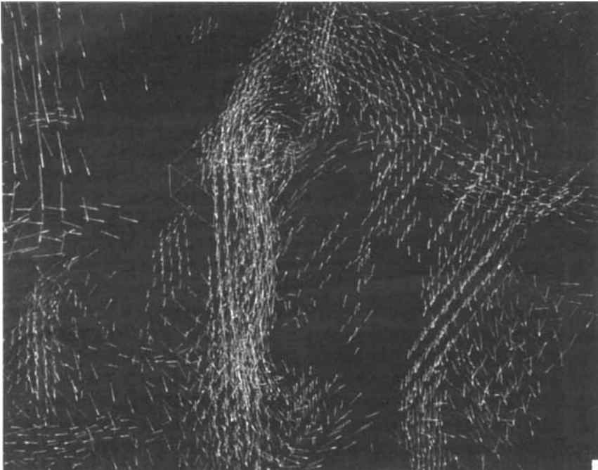
FIGURE 2. (a) Detail of the vorticity field showing two approximately parallel tubes; with a secondary counter-rotating tube between them. (b) The same vorticity region as (a) one turnover time later. The three vorticity tubes of (a) have merged into one larger tube.
