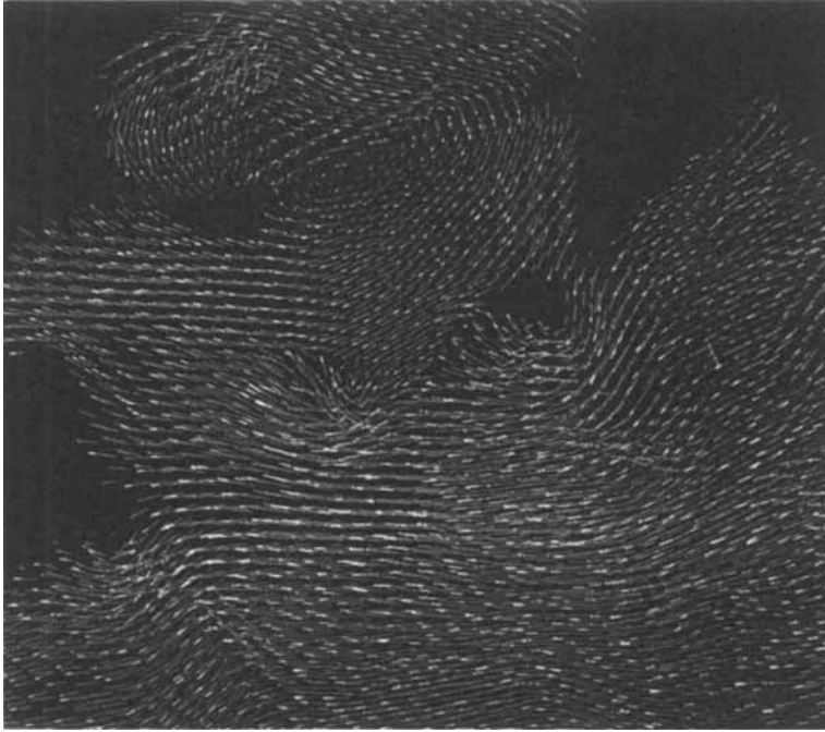
FIGURE 3. The velocity field in a plane approximately perpendicular to the vorticity tubes.
